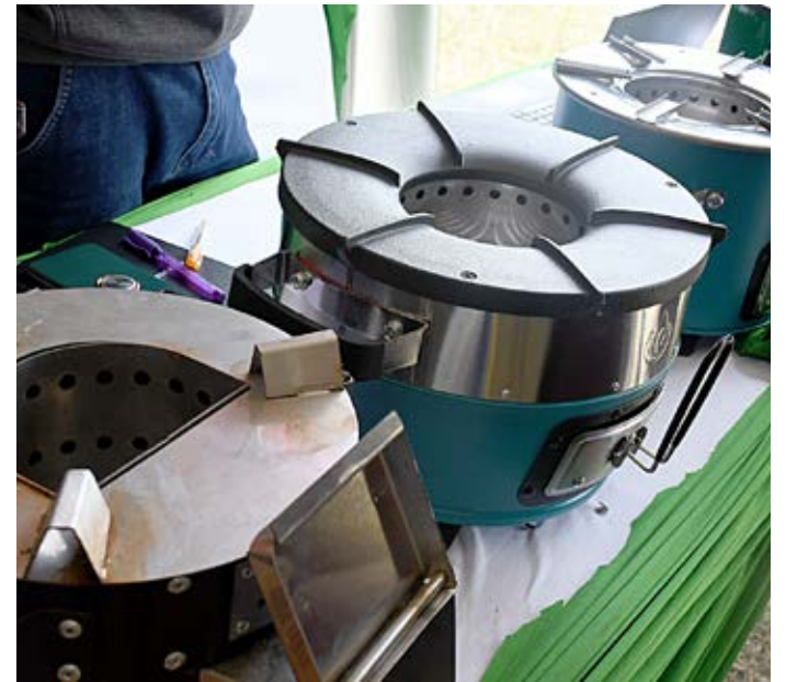
Modern Eco-Friendly Jikos by Lowaki Eco-Solutions Limited, using briquettes and charcoal. (Photo: Yvonne Wangeci)
