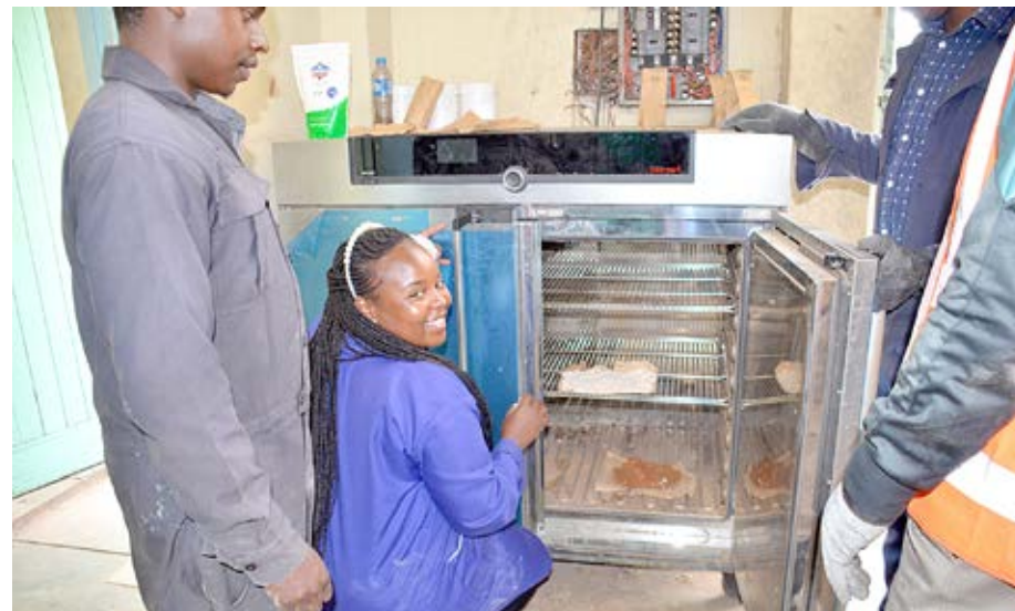
Geologists drying a wet rock in a giant rock oven before the crushing process at the Madini Lapidary lab
