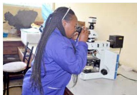
A geologist at Madini lab conducting a petrographic analysis on a rock fragment.
